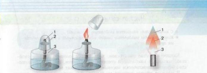
The diagram consists of two parts. On the left, labeled 'Рис. 5', is a spirit lamp with three numbered parts: 1 (wick), 2 (cap), and 3 (reservoir). On the right, labeled 'Рис. 6', is a diagram of a flame with three numbered zones: 1 (outermost, colorless), 2 (middle, yellow), and 3 (innermost, blue).
